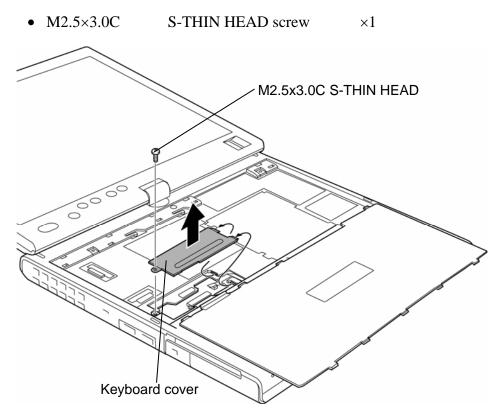
Figure 4-16 Removing the keyboard cover
